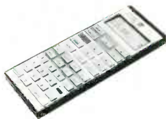
GE CONTROL CENTRAL programmable remote system
