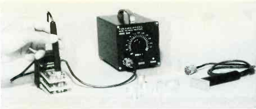
FIG. 23—THERMO-PROBE CAN SUPPLY PRECISELY-CONTROLLED TEMPERATURE. The production-line model is shown here; a test-bench model is also available.
