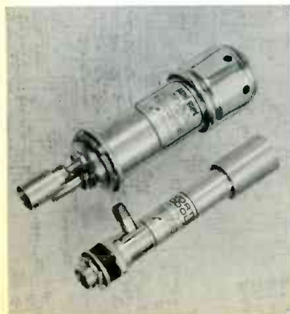
FIG. 27—A THERMOSTAT may be an integral part of a vortex tube.
