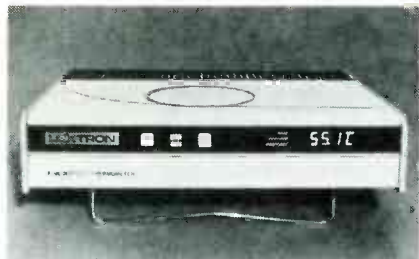
FIG. 17—LUXTRON'S FLUOROPTIC THERMOMETER has both analog and digital outputs for peripheral devices.
