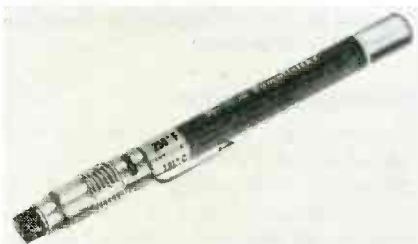
FIG. 15—THIS "TEMPILSTIK"™ changes color at 121°C.
